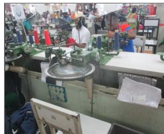
Photo of non-conformity No needle cover was not found in linking machine.JPG
